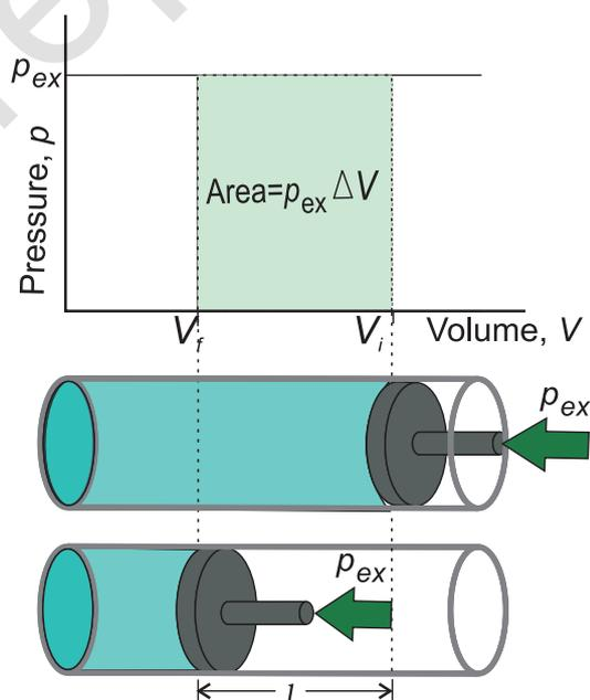
**Fig. 6.5(a)** Work done on an ideal gas in a cylinder when it is compressed by a constant external pressure,  $p_{ex}$  (in single step) is equal to the shaded area.
