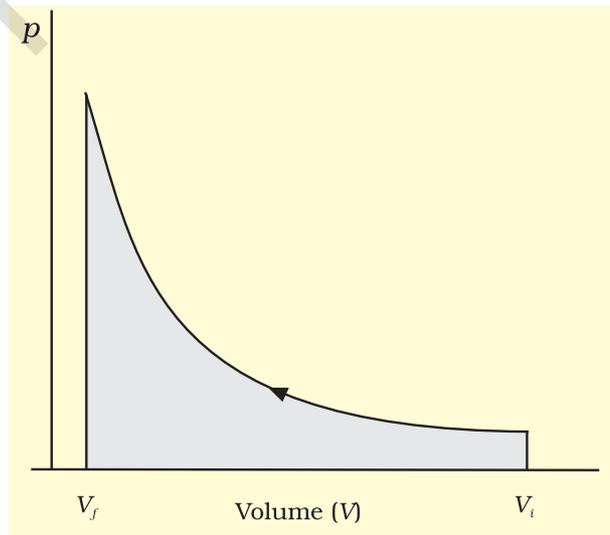
**Fig. 6.5 (c)**  $pV$ -plot when pressure is not constant and changes in infinite steps (reversible conditions) during compression from initial volume,  $V_i$  to final volume,  $V_f$ . Work done on the gas is represented by the shaded area.
