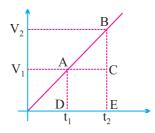
Total distance travelled by body between  $t_2$  and  $t_1$ , time intervals
