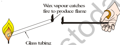
Fig. Dark inner zone contains unburnt wax vapour
