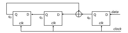
The following data: 100110000 is supplied to the "data" terminal in nine clock cycles. After that the values of  $q_2q_1q_0$  are:
