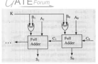
If the operands are in 2's complement representation, which of the following operations can be performed by suitably setting the control lines K and  $C_0$  only (+ and - denote addition and subtraction respectively)?
