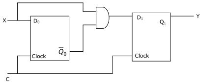
Consider the following timing diagrams of X and C; the clock period of  $C \ge 40$  nanosecond. Which one is the correct plot of Y?
