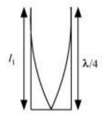
Such a system produces odd harmonics. The fundamental note in a closed pipe is given by the relation:
