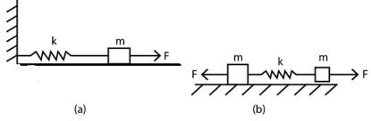
Figure (a) attached shows a spring of force constant k clamped rigidly at one end and a mass m attached to its free end. A force F applied at the free end stretches the spring. Figure (b) shows the same spring with both ends free and attached to a mass m at either end. Each end of the spring in Fig. (b) is stretched by the same force F.
