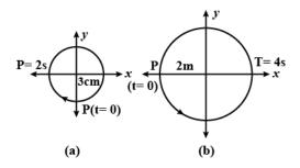
Figures given correspond to two circular motions. The radius of the circle, the period of revolution, the initial position, and the sense of revolution (i.e. clockwise or anticlockwise) are indicated on each figure. Obtain the corresponding simple harmonic motions of the x-projection of the radius vector of the revolving particle P, in each case.
