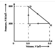
A thermodynamic system is taken from an original state to an intermediate state by the linear process shown in the figure.
