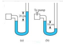
A manometer reads the pressure of a gas in an enclosure as shown in Fig (a). When a pump removes some of the gas, the manometer reads as in Fig (b). The liquid used in the manometers is mercury and the atmospheric pressure is 76 cm of mercury.
