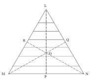
concurrence of the median, i.e. on the centroid G of the triangle. Thus centroid of the triangle itself is the centre of mass of the triangular lamina.
