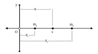
Let 'C' be the centre of mass of the system which is at a distance X from the origin O.
