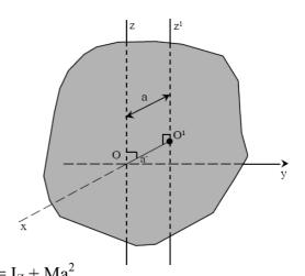
Where  $I_Z$  and  $I_z^{-1}$  are the moments of inertia of the body about the Z and Z axes respectively, M is the total mass of the body and  $\boldsymbol{a}$  is the perpendicular distance between the two parallel axes.
