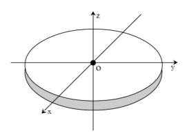
Consider three concurrent axis through the centre of the disc, O as the x, y, z axes.
