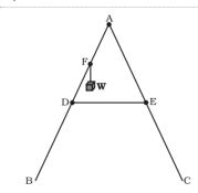
As shown in Fig., the two sides of a step ladder BA and CA are 1.6 m long and hinged at A. A rope DE, 0.5 m is tied half way up. A weight 40 kg is suspended from a point F, 1.2 m from B along the ladder BA. Assuming the floor to be frictionless and neglecting the weight of the ladder, find the tension in the rope and forces exerted by the floor on the ladder. (Take  $g = 9.8 \text{ m/s}^2$ ) (Hint: Consider the equilibrium of each side of the ladder separately.)
