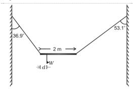
A non-uniform bar of weight W is suspended at rest by two strings of negligible weight as shown in Fig. The angles made by the strings with the vertical are  $36.9^{\circ}$  and  $53.1^{\circ}$  respectively. The bar is 2 m long. Calculate the distance d of the center of gravity of the bar from its left end.
