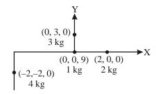
$$\begin{array}{ll} \therefore & I = \ I_1 + I_2 + I_3 + I_4 \\ & = \ 0 + 0 + 27 + 16 = 43 \ kg \ m^2 \end{array}$$
