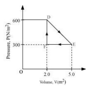
Its volume is then reduced to the original value from E to F by an isobaric process. Calculate the total work done by the gas from D to E to F
