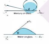
In the diagram  $S_{SL}$ ,  $S_{LA}$  and  $S_{SA}$ , are the respective interfacial tensions between the liquid-solid, liquid-air, and solid-air interfaces. At the line of contact, the surface forces between the three media are in equilibrium, i.e.,
