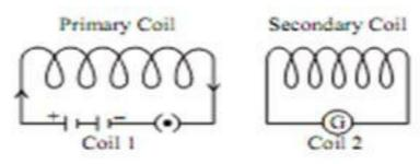
In this experiment plug in the key that connects coil with battery and observe the deflection in galvanometer. Now plug out the key that disconnect the coil-1 from battery and observe the deflection in galvanometer, which will be in reverse direction.
