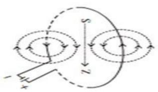
Every point on the wire carrying current give rise to the magnetic field, appearing as a straight line at the centre of loop. By applying Right hand Thumb rule, we can find the direction of magnetic field at every section of the wire.
