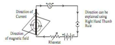
Let a current carrying conductor be suspended vertically and the electric current is flowing from south to north. In this case, the direction of magnetic field will be anticlockwise. If the current is flowing from north to south, the direction of magnetic field will be clockwise.
