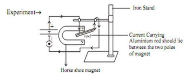
We will observe that the rod will displace i.e. the rod will experience a force, when it is placed in magnetic field, in a perpendicular direction to its length.
