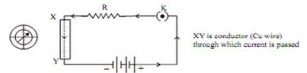
On passing the current through the copper wire XY in the circuit, the compass needle which is placed near the conductor gets deflected. If we reverse the direction of current, the compass needle deflect in reverse direction. If we stop the flow of current, the needle comes at rest.
