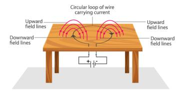
For the downward direction of the current, the direction of the magnetic field will be as if emerging from the table outside the loop and merging the table inside the loop. Similarly, for current flowing in the upward direction, the direction of the magnetic field will as if they are emerging from the table outside the loop and merging to the table inside the loop as shown in the figure.
