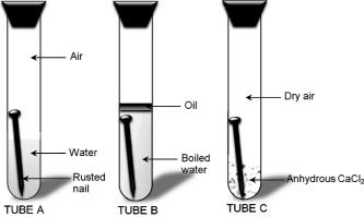
**Observation:** Iron nails get rusted in test tube A because both air and water are present in it. Iron nails do not get rusted in B because there is water but no air. In C, rusting will not take place because there is neither air nor water. Conclusion: Iron gets rusted in the presence of air and water.
