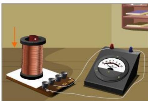
The South Pole of the Magnet is Moved into the Coil of Wire
