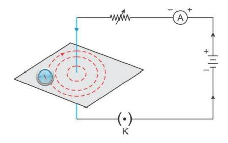
• The direction of a magnetic field is given by the **Right-Hand Thumb Rule**.
