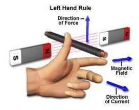
Arrange your fingers of left hand such that the fore finger points towards the direction of magnetic field and centre finger shows the direction of current, then the thumb will show the direction of force or motion.
