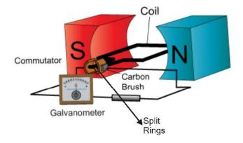
**Note:** The only difference between an AC and a DC generator is in the way the two ends of generator coil are linked to the outer circuit.
