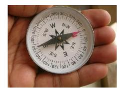
It is an instrument consisting of base and a needle. The needle has north and south tip whose north tip is painted red (generally). The needle gets deflected when close to magnet and it gives the direction of Magnetic field.
