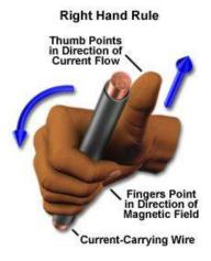
**Right hand thumb rule** states that if we hold the current carrying wire in the right hand and if the thumb points towards the current, the direction in which the fingers encircle gives the direction of Magnetic field.
