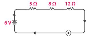
2. Redraw the circuit of Question 1, putting in an ammeter to measure the current through the resistors and a voltmeter to measure the potential difference across the 12  $\Omega$  resistor. What would be the readings in the ammeter and the voltmeter? Solution:
