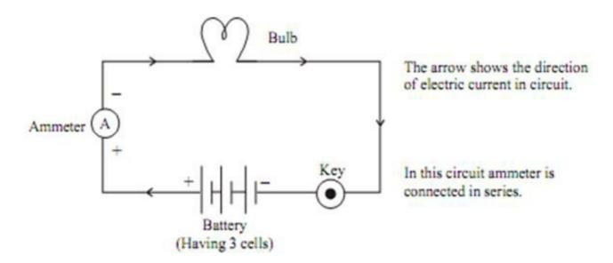
The electrons can only flow when there is difference of electric potential. For example "water flowing through a tube". It is only possible when there is high pressure at one side and low at another side, then it will move from high pressure to low pressure.
