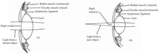
Fig. 28.13 Focussing and accomodation of the eye a) Distant object b) Near object
