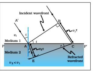
$$\therefore \quad \frac{\sin i}{\sin r} = \frac{BC/AC}{AE/AC} = \frac{BC}{AE} = \frac{v_1\tau}{v_2\tau} = \frac{v_1}{v_2}$$
