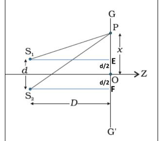
$$\therefore (S_2 P)^2 - (S_1 P)^2 = \left[ D^2 + \left( x + \frac{d}{2} \right)^2 \right] - \left[ D^2 + \left( x - \frac{d}{2} \right)^2 \right]$$
