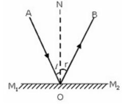
• **Formation of Image by the Plane Mirror:** The formation of image of a point object O by a plane mirror is represented in figure.
