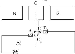
NS - Field Magnet - used for producing magnetic field, usually electromagnet.
