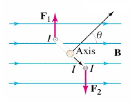
→ When loop is vertical, current switches sign and the forces reverse, in order to keep the loop in rotation.
