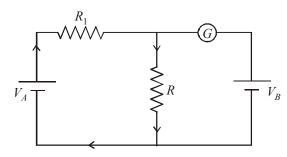
Since deflection in galvanometer is zero so current will flow as shown in the above diagram.
