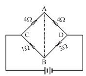
Potential drop over the resistance CA will be more due to higher value of resistance. So potential at A will be less as compared with at B. Hence, current will flow from B to A.
