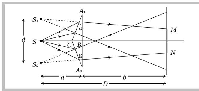
Let the separation between  $S_1$  and  $S_2$  be  $d$  and the distance of slits and the screen from the biprism be  $a$  and  $b$  respectively *i.e.*  $D = (a + b)$ . If angle of prism is  $\alpha$  and refractive index is  $\mu$  then  $d = 2a(\mu - 1)\alpha$
