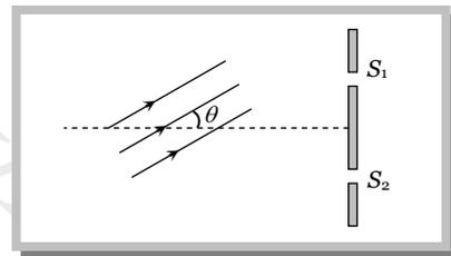
137. In a Young's double slit experiment, let  $\beta$  be the fringe width, and let  $I_0$  be the intensity at the central bright fringe. At a distance  $x$  from the central bright fringe, the intensity will be
