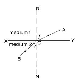
Where  $_{a}\mu_{b}$  is a constant known as **Refractive Index** of the medium b with respect to the medium a ; i is the angle incidence in medium a and r is the angle of refraction in medium b.
