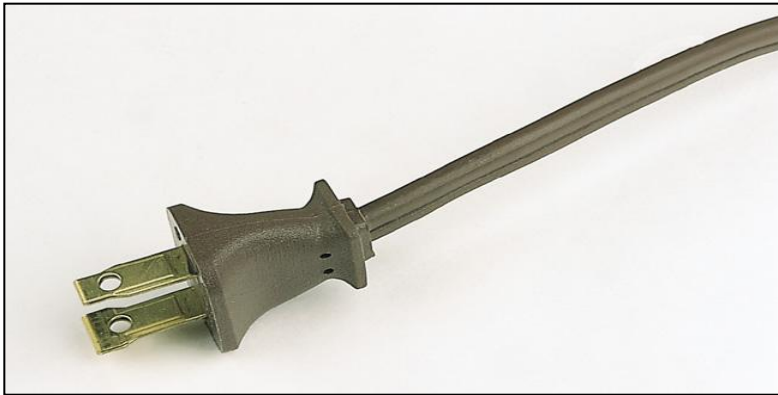
Fig. 15-22: Plug connectors polarized for ground connection to an ac power line. (a) Wider blade connects to neutral. (b) Rounded pin connects to ground.
