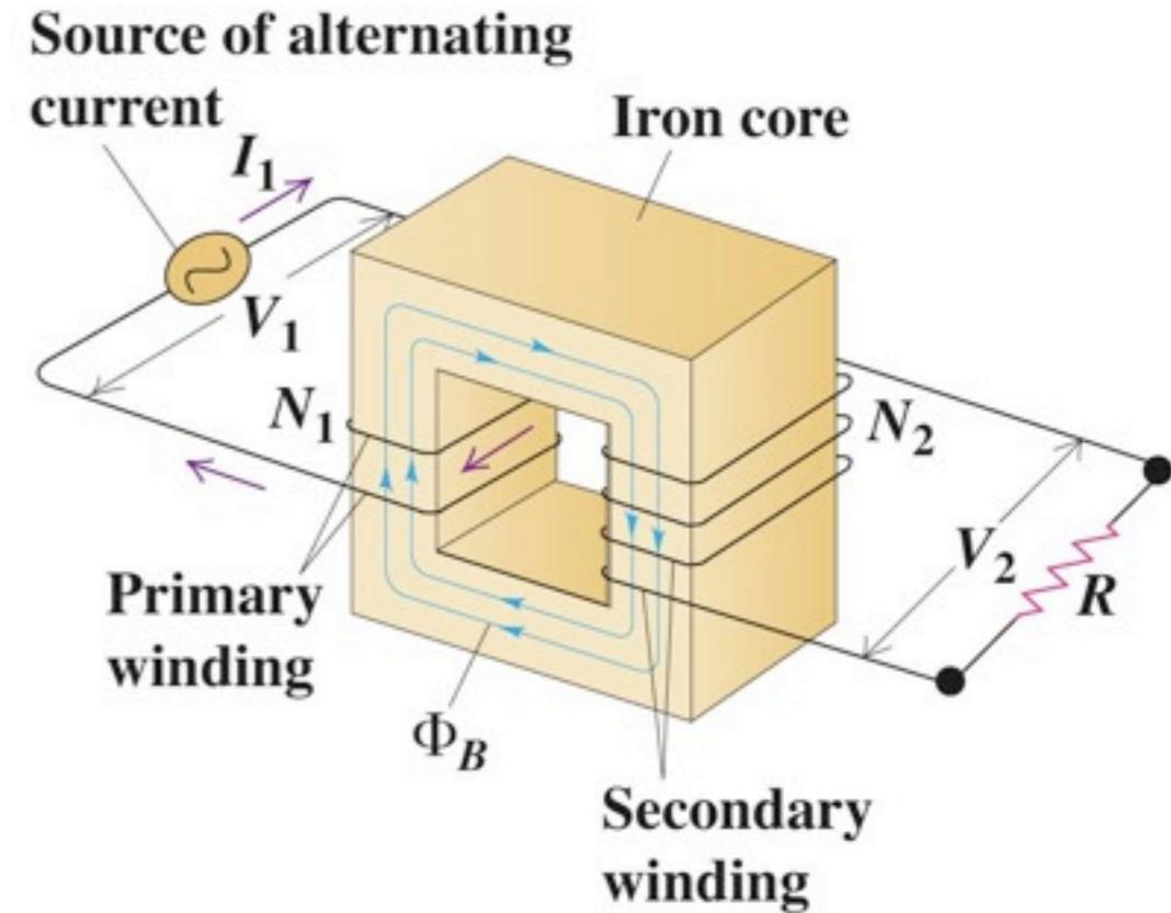
→  $N_2 > N_1 : V_2 > V_1$  - a “step-up” transformer
