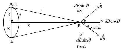
Consider a coild of radius R carrying current i ampere in the anticlockwise direction A and B are two current elements of length dl at the diametrically opposite edges of the coil. Magnetic field at P due to A
