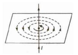
The direction of magnetic field lines can be obtained by Right Hand Thumb Rule
