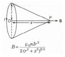
where, r = radius of the coil, n = number of turns in the coil and I = current,
