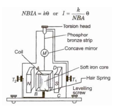
where, k = restoring torque per unit twist,
