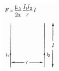
The force is attractive if current In both conductors is in same direction and repulsive if current 10 both conductors is in opposite direction.
