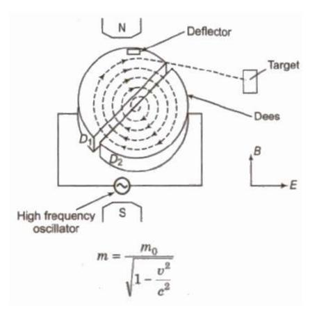
Where, m = mass of the lOD.  $m_o = maximum$  mass of the ion. v = speed of Ion and c = speed of light.
