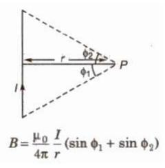
where  $\varphi 1$  and  $\varphi 2$  are angles, which the lines joining the two ends of the conductor to the observation point make with the perpendicular from the observation point to the conductor.
