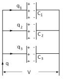
When capacitors are connected in parallel, the potential difference V across each is same and the charge on  $C_1$ ,  $C_2$  and  $C_3$  is different i.e  $q_1$ ,  $q_2$  and  $q_3$ The total charge q is given by
