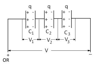
Capacitor are said to be connected in series if charge on each individual capacitor is same. In this situation
