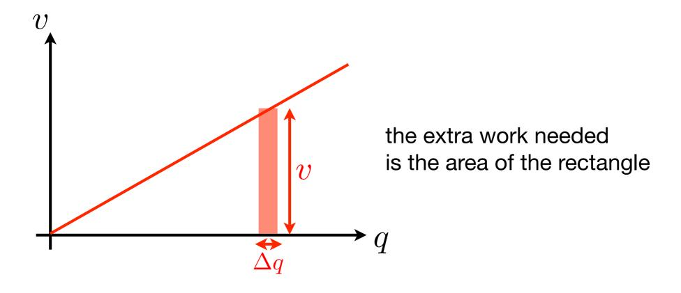
getting the charges in place on the plates requires work - this work ends up as energy 'stored' in the electric fields
