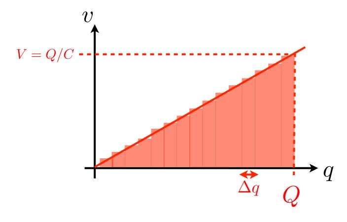
the total work required is the area under the curve  $W = \frac{1}{2} \times Q \times \frac{Q}{C} = \frac{Q^2}{2C}$  $W = \frac{1}{2}CV^2$
