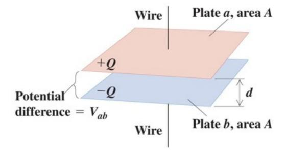
(a) A basic parallel-plate capacitor
