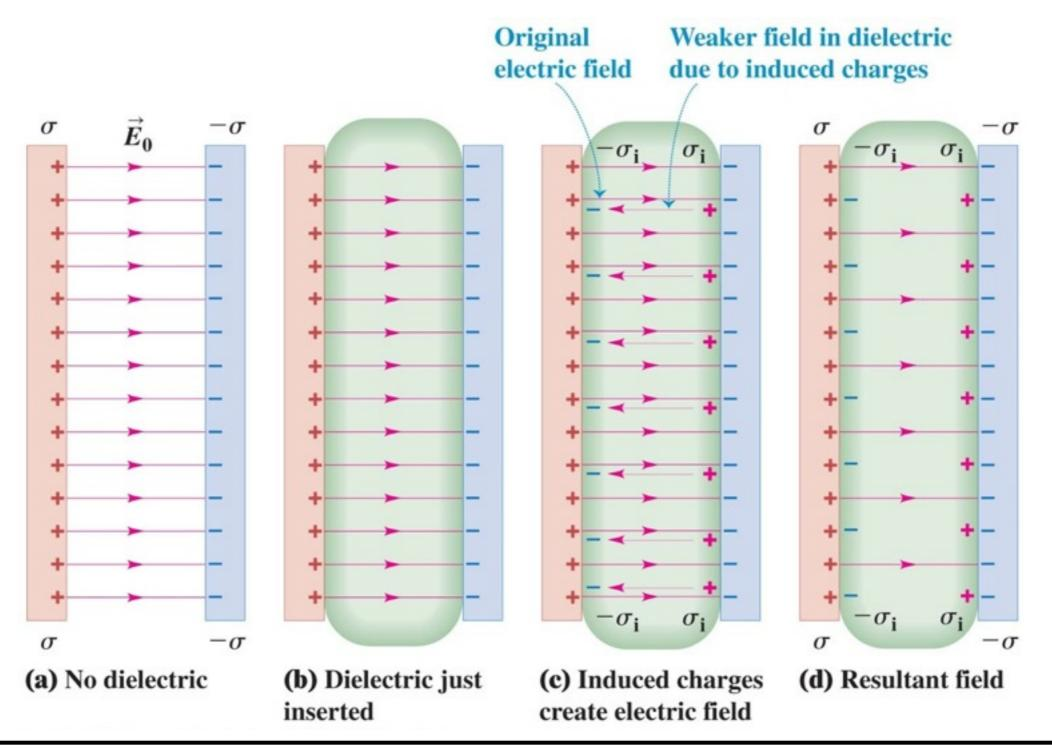
→ the induced charge is caused by the polarization of electric dipoles in the dielectric
