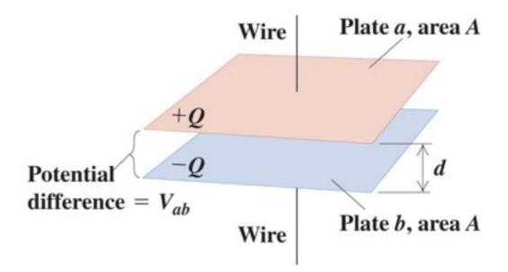
(a) A basic parallel-plate capacitor
