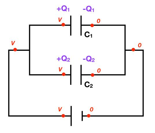
$$Q_1 = C_1 V \qquad Q_2 = C_2 V$$
