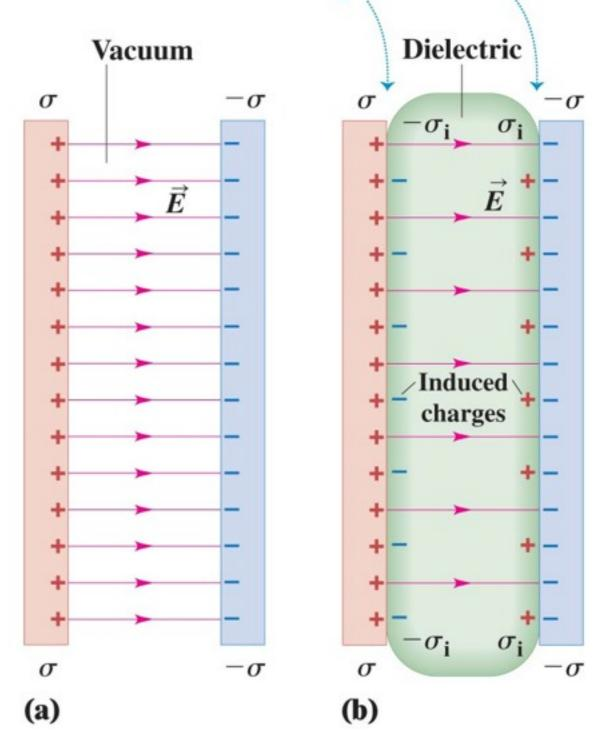
→ the voltage drop corresponds to a reduction of the electric field in the gap
