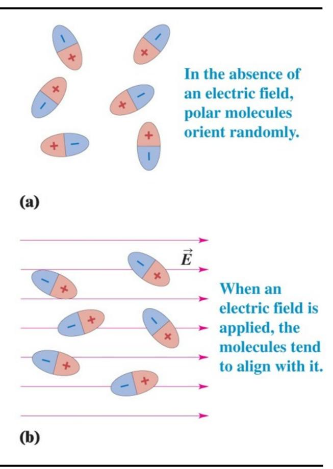
→ the induced charge is caused by the polarization of electric dipoles in the dielectric
