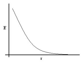
Coulomb's law: The mutual electrostatic force between two point charges q<sub>1</sub> and q<sub>2</sub> is proportional to the product  $q_1q_2$  and inversely proportional to the square of the distance  $r_{21}$  separating them.
