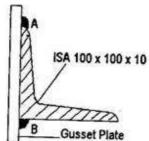
2.7 ISA  $100 \times 100 \times 10$  mm (Cross sectional area = 1908 mm 2) serves as tensile member. This angle is welded to a gusset plate along A and B appropriately as shown. Assuming the yield strength of the steel to be 260 N/ mm2 the tensile strength of this member can be taken to be approximately,
