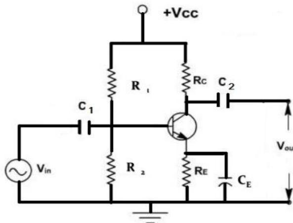
4. For the CE amplifier circuit using silicon transistor given below, find
