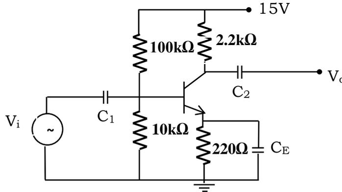
5. CE amplifier circuit using Germanium transistor is shown in figure, calculate
