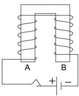
The diagram shows a coil wound around a U shape soft iron bar AB.
