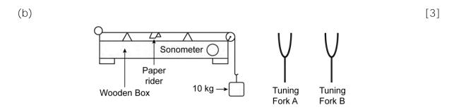
The diagram above shows a wire stretched over a sonometer. Stems of two vibrating tuning forks A and B are touched to the wooden box of the sonometer. It is observed that the paper rider (a small piece of paper folded at the centre) present on the wire files off when the stem of vibrating tuning fork B is touched to the wooden box but the paper just vibrates when the stem of vibrating tuning fork A is touched to the wooden box.
