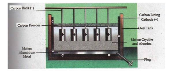
• The carbon blocks in this cell are replaced from time to time because the O<sub>2</sub> liberated in the anode is oxidising the Carbon rod and produce carbon dioxide.
