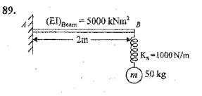
The fundamental time period of vibration of the system shown in the figure, by neglecting the self weight of the beam, is nearly
