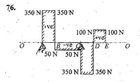
The shear force diagram of a single overhanging beam is shown in figure. One simple support is at end A. The 'total' downward load acting on the beam is,
