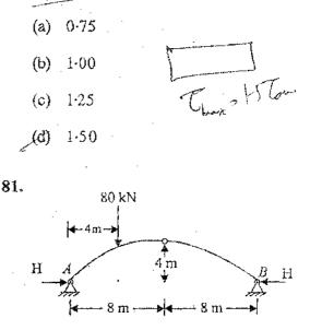
The horizontal thrust of the three-hinged arch loaded as shown in the figure is
