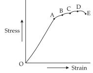
• The stress is proportional to strain upto point, where, Hooke's law is fully obeyed. Point A is known as proportional unit.
