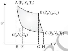
(i) First Step : Isothermal expansion curve AB. The cylinder with gas is allowed to expand slowly at constant temperature T<sub>1</sub> by putting in on the source.
