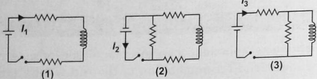
Rank the circuits according to the currents through the battery just after the switch is closed, in descending order.
