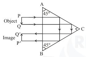
Topic: Refraction of light at plane surfaces\_Subtopic: Total internal reflection through a prism\_ Level: Medium Std. X ICSE Board / Physics
