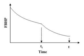
Let k is the reservoir permeability, h is the formation thickness and  $\mu$  is the viscosity of the oil.  $\Delta P_D(t)$  is constant-rate dimensionless pressure drop as a function of time. The total pressure drop till time, t, where  $t > t_1$ , will be:
