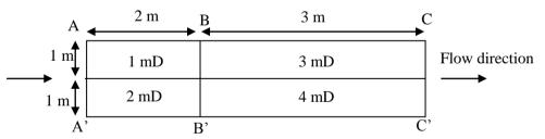
The pressure at the cross-sections AA', BB', and CC' is 2 bar, 1.5 bar, and 1 bar, respectively. The permeability in mili-Darcy and lengths AB and BC in meters are given in the figure. The effective permeability of the rock from AA' to CC' is \_\_\_\_mD. (rounded-off to two decimal places)
