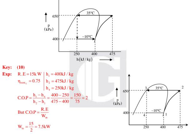
: Isotropic efficiency of compressor is given, actual compressor power required
