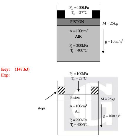
Total pressure on the piston =  $P_{\infty}$  + pressure due to weight of piston
