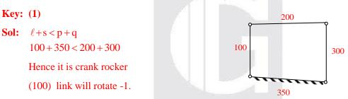
So, link whose length is 100 mm will rotate fully. So, only one link will rotate fully.
