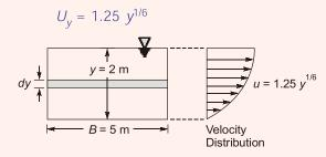
Discharge through elementary strip  $(dQ) = 5dy \times u$
