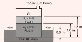
Unit weight of water,  $\gamma_w = 9.81 \text{ kN/m}^3$ Atmospheric Pressure,  $p_{\text{atm}}$  = 95.43 kPa
