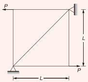
For the loads shown on the truss, the statement that correctly represents the nature of forces in the members of the truss is:
